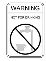
EVERY EXTERNAL SUPPLY OUTLET FROM RAINWATER RE-USE TANK TO BE LABELED WITH METALLIC WARNING SIGN
