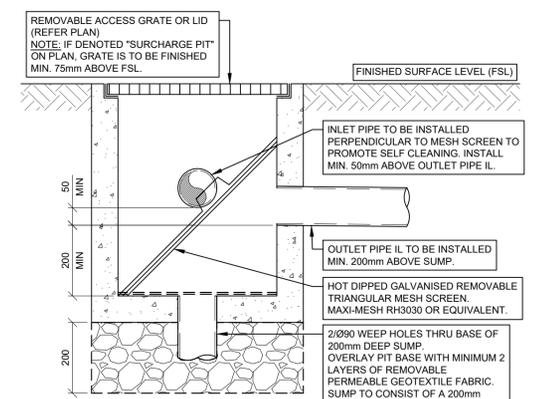
TYPICAL SILT ARRESTOR PIT DETAIL
