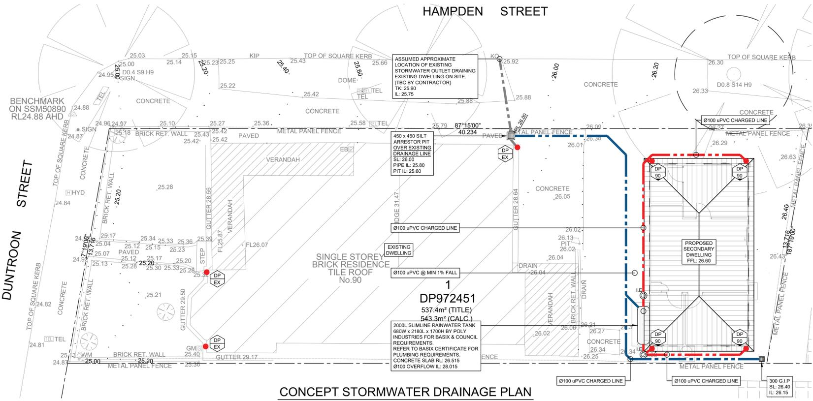
CONCEPT STORMWATER DRAINAGE PLAN
